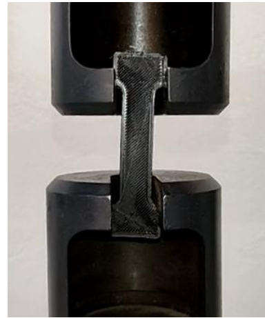
Figure 8. Gripping system of testing machine.
